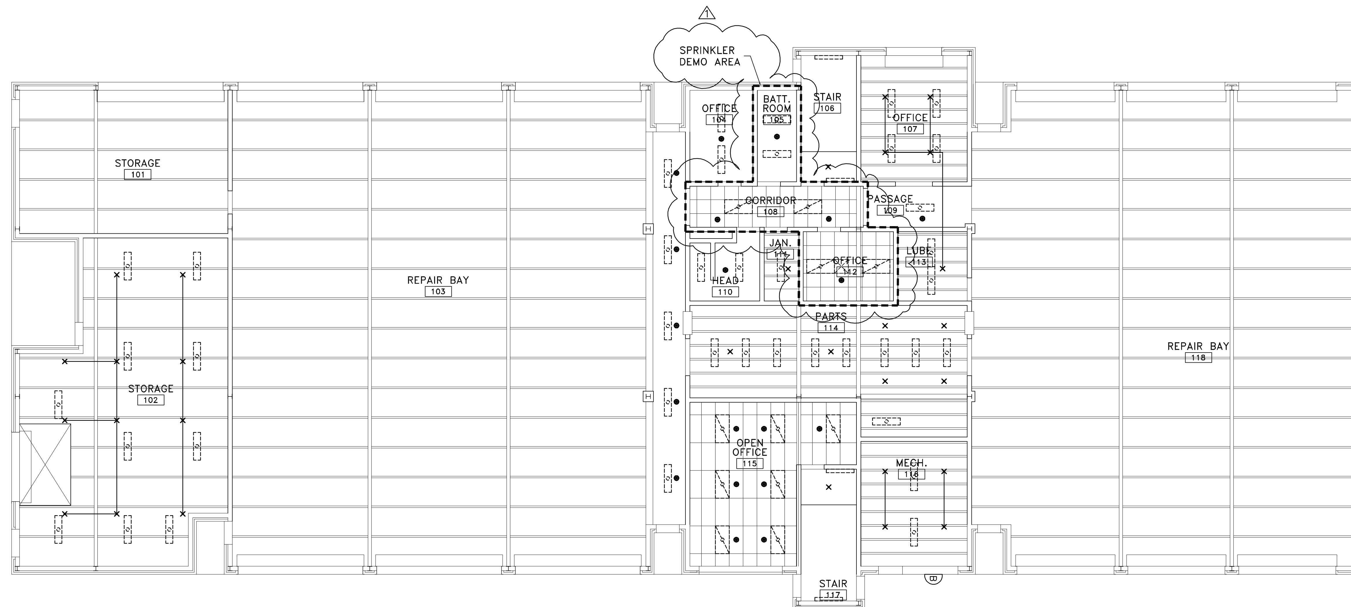
A FIRE PROTECTION DEMOLITION 1ST FLOOR PLAN 1/8" = 1'-0"
